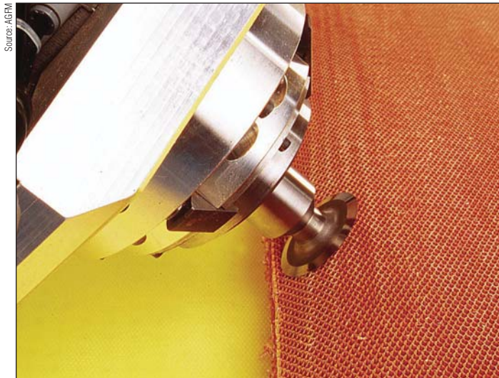
Source: AGFM Six-axis ultrasonic cutter incorporates a disc to sculpt honeycomb air foil shape.
